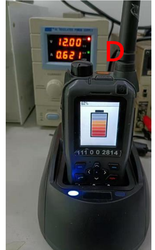
Charge 3.5hr, radio LED flashing Green. Power guage 62%
