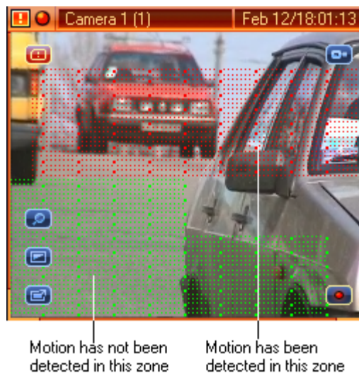
Figure 106. Camera cell with alarmed zone
