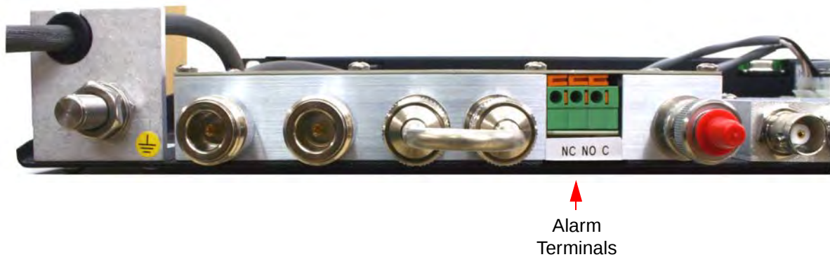
Figure 13: Alarm terminals. Normally open and normally closed terminals are available.
